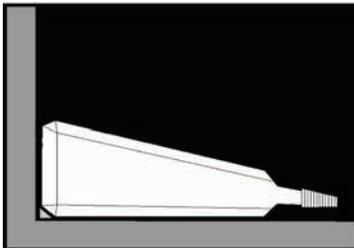
**Note:** Beveled edges are designed to function as a squeegee and must face direction of excess silicone removal. Small corner beveled edge pushes silicone into gap and leaves proper amount of silicone. If larger silicone bead is necessary, cut small corner beveled edge to desired shape to allow for more silicone and a larger bead.
