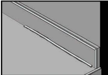
1.) Place small bead of Silicone in joint. Bead should be approximately 1/8" x 1/8" to avoid waste.
