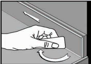
3.) Place longest beveled edge of the PERFECT BEAD TOOL on the horizontal surface and rotate small tip in direction of excess silicone removal.
