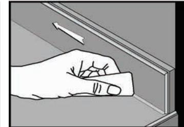
5.) Using moderate pressure, move the PERFECT BEAD TOOL along silicone normally with one pass. Intermittent removal of excess silicone from tool is suggested for best performance. If smoother silicone bead is required repeat steps 2 through 5.
